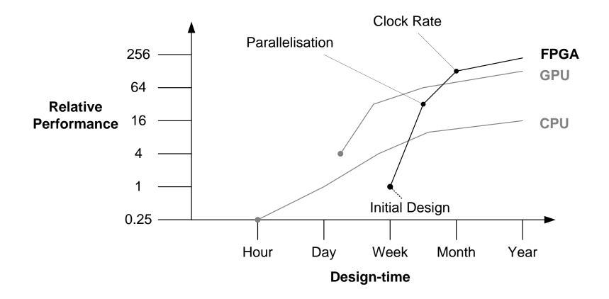
FPGAs provide large speed-up and power savings – *at a price!* Days or weeks to get an initial version working Multiple optimisation and verification cycles to get high performance
